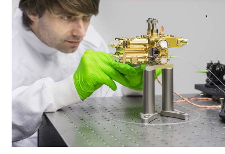
The possibilities of quantum technologies are so great that they could have major effects on our economy and society, and are furthermore extremely relevant to security policy. The image shows one example: a single photon source for inherently secure data transmission. The international race to turn these technologies into industrial reality has already begun.
