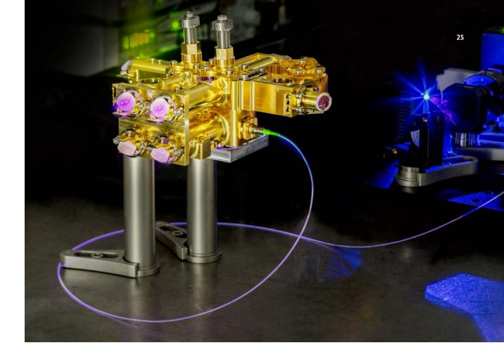
Technological approaches to quantum key exchange are primarily based on photonics. The fundamental reason for this is that not only can photons (light particles) be generated and prepared with comparatively low technological costs, they can also be transported over large distances without losing their quantum characteristics. Single photon sources (such as those shown in the image) are used to generate these specially prepared photons.
